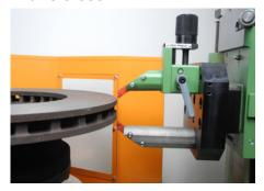
Brake discs of any size can be mounted in the three-jaw chuck and finely turned on both sides simultaneously with the double toolholder.
