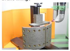
The U 305 is also suitable for skimming brake linings as well as for facing cylinder heads by turning and grinding.
