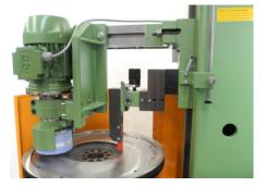
The turning or grinding of the clutch face on small or large flywheels presents no problem. The workpieces are gripped quickly and accurately in the three-jaw chuck.
