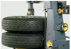
With the U 305 also brake drums with complete mounted sets of wheels can be operated. Necessary therefore is the long swivel arm.
