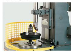
Usually brake drums are just turned. This can be carried out either in the upward or downward direction using the automatic feed. For instance, a downward roughing cut and an upward
