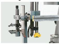
The 2 station tool changer keeps toolholders and other equipment ready for use.
