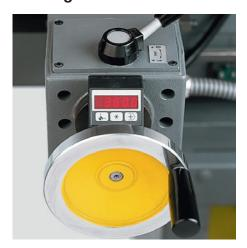
For rapid and precise adjustment of the drum turning diameter and the rotation speed LCD digital read-outs can be incorporated.
