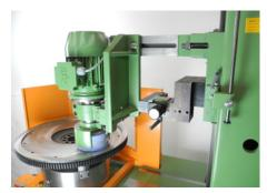
The surface grinding attachment for cross-hatch grinding attaches to a special support on the long swivel arm.
