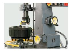
finishing cut can be employed. It is, of course, also possible to grind the brake drums either subsequent to turning or simultaneously with it.
