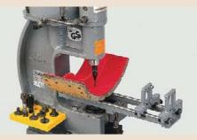
With all riveting machines marketed hither to, it has been necessary to insert the rivets individually from below into the lining and prevent them by hand from dropping out. With the newly developed HUNGER device, the riveting punch is at the bottom and the riveting dolly at the top (top photo).
