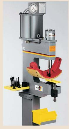
The N 332/80-CE has an extended stroke of 80 mm and a threat clearance of 230 mm. It is especially suited to the handling of brake shoes with double webs. The extended throat permits the riveting of the rear line of holes without turning the brake shoes.
