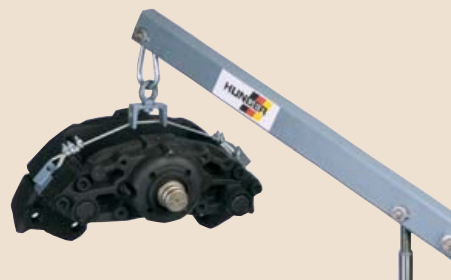
Lifting tackle for calipers.
